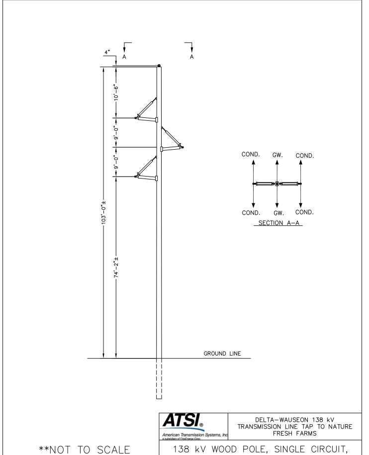
138 kV WOOD POLE, SINGLE CIRCUIT, BRACE POST INSULATOR, DELTA TANGENT
