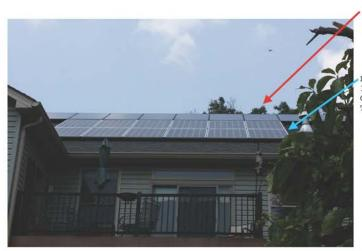
Original Array 12 panels (top row): SW225 Orientation: 135 Tilt: 30.26
