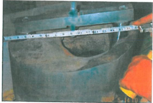
The hole in the Davis-Besse reactor head, 2002
