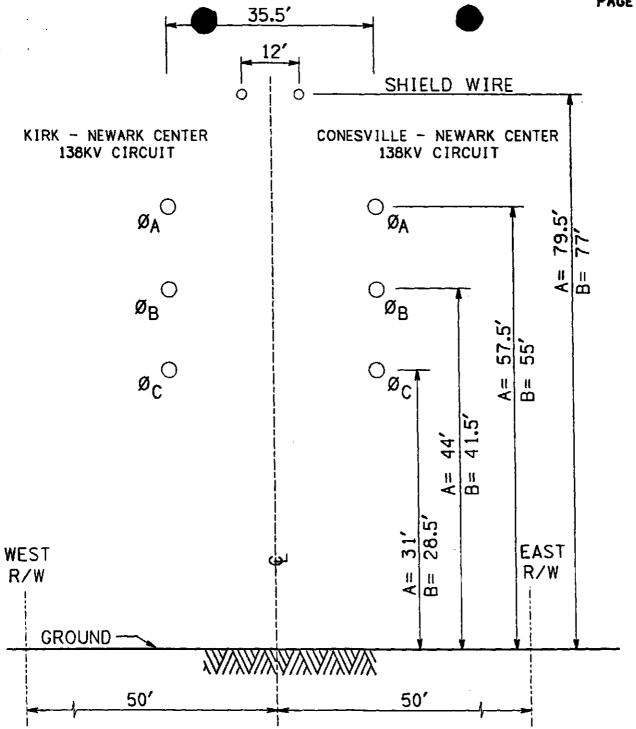
DIMENSION "A" - DOUBLE CIRCUIT - VERT. CONFIGURATION (UNDER EMERGENCY & NORMAL MAX. LINE LOADING) DIMENSION "B" - DOUBLE CIRCUIT - VERT. CONFIGURATION
