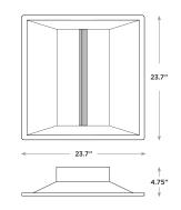
NOTE: Use of Expanded Junction Box will expand the depth to 6.67" and Emergency Backup will expand the depth to 6.30".
