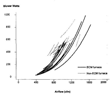
Figure 2: Blower power versus airflow curves for study furnaces.
