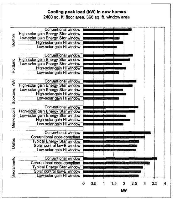
According to our estimates, low-solar-gain HI windows reduce peak cooling load by an average 28 percent if compared with conventional windows across different climates. Even high-solar-gain HI windows would achieve an average peak load reduction by 18 percent.
