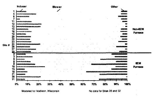
Figure 17: Heating-mode electricity use by cycle phase.
