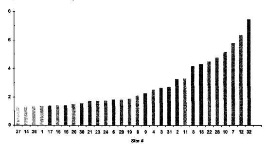
The number of heating cycles that a furnace goes through in a day is strongly correlated with outdoor temperature for most of the sites (see Appendix C). Indeed it appears that, for the most part, it is more the increase in the number of heating cycles rather than the length of the heating cycle that contributes to the increase in total furnace run time as the outdoor temperature drops.
