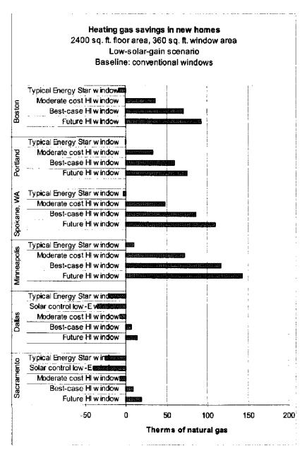
High performance windows can lead to more heating energy use if they block a substantial fraction of solar heat gain. This is particularly obvious in climates with strong solar heat even in wintertime.
