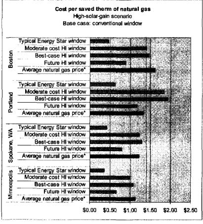
Figure 4: Heating gas savings in new homes with high-solar-gain high-performance windows Base case: Conventional windows
