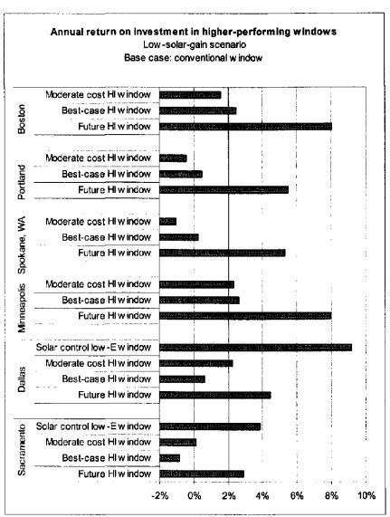
In heating-dominated climates, windows designed for low solar gain are not estimated to provide as high energy savings as windows designed for high solar gain. Nevertheless, low-solar-gain windows can provide substantial cooling peak load reductions and allow for HVAC system downsizing (see Figure 5).
