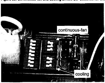
Figure 30: Continuous-fan and cooling airflow DIP switches for Site 2.
