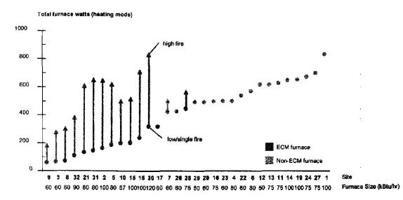
Figure 4: Heating mode power draw.
