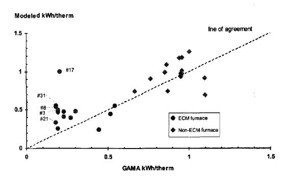
Figure 14. Modeled versus rated heating kWh per therm.
