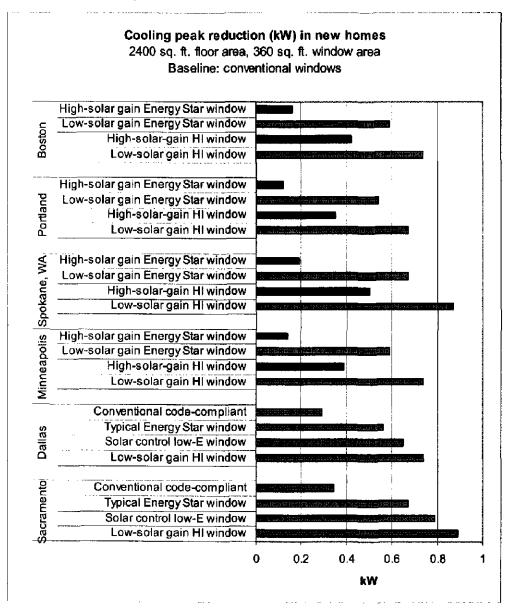
Figure 9: Cooling electricity savings in new homes depending on window type (low-solar-gain windows marked blue)
