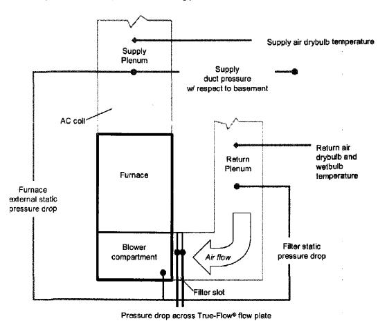
Figure 1: Static pressure and temperature monitoring points.
