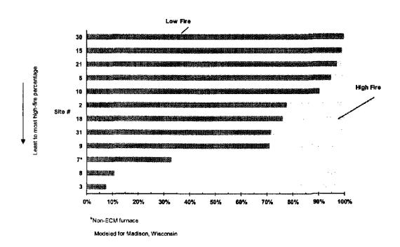
Figure 9: Low/High-fire proportions for two-stage furnaces.
