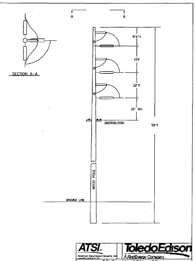
DELTA-WAUSEON 138kV TRANSMISSION LINE TAP TO ZINC OX 3-WAY DEAD END W/DISC. TAPS STRUCTURE
