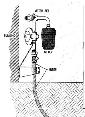
This drawing shows the most common type of riser installation for new homes – details of your riser installation may vary.
