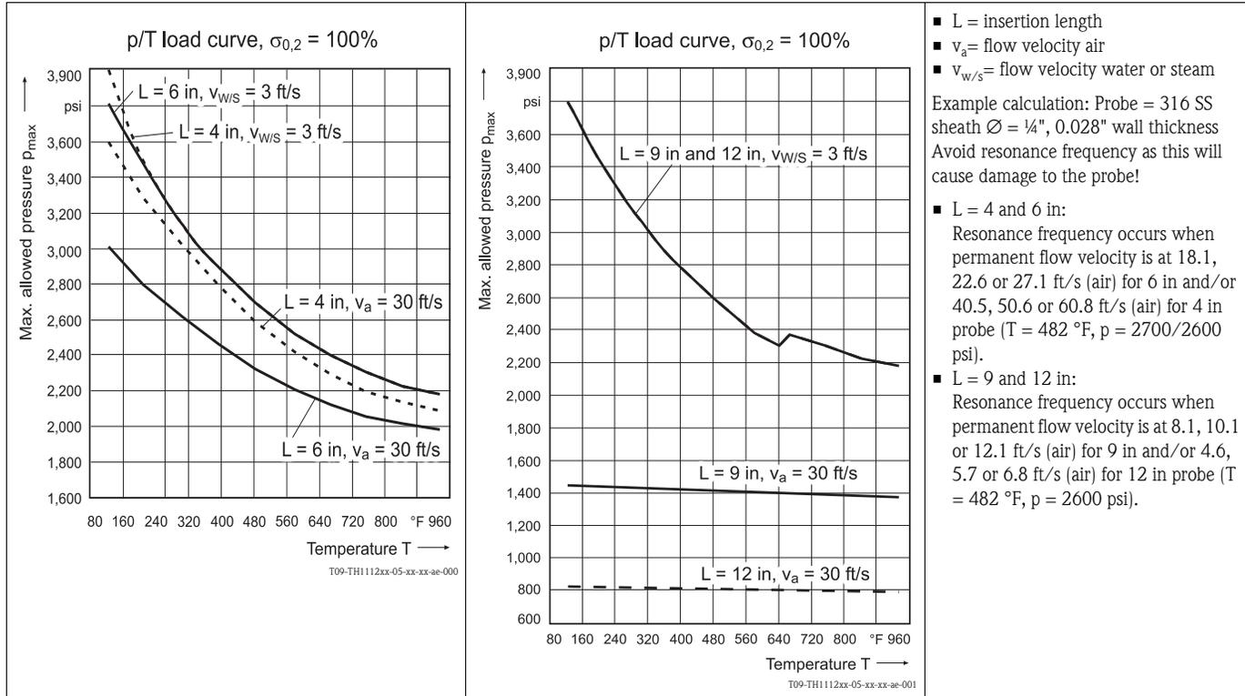
Max. allowable process pressure (PSIG) for instrumentation with one time adjustable compression fittings.
